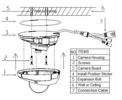
Step one: Measure the height of installation on wall and mark the holes positions.
